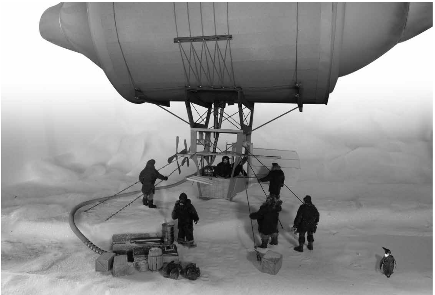
Hurt gives instructions to several unidentified crew members. First Mate, Federico Lawrence, is at the rudders. Hydrogen for the craft was produced from sulfuric acid, iron filings and sea water. The dual propellers driven by a Franz Kravogl electric motor.
